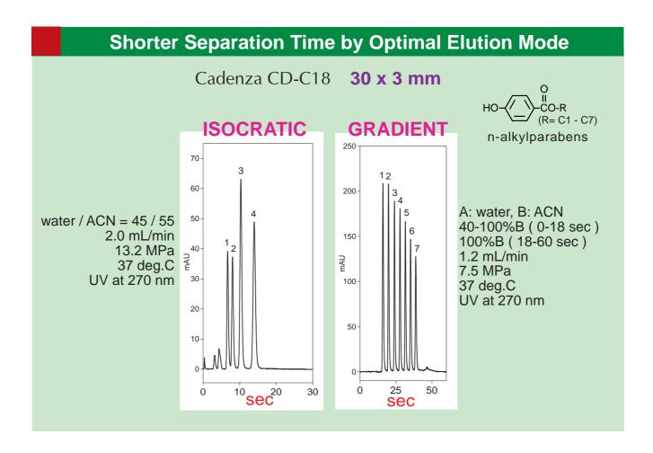
This is an elution mode comparison of high-speed separation by the small column Cadenza CD-C18.
