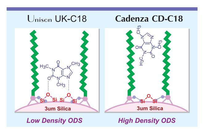
Unison UK-C18 has a slightly lower ODS ligand density compared to Cadenza CD-C18. As a result, highly polar substances such as caffeine tend to have longer retention times due to electrostatic interactions with the oxygen atoms of the siloxane (Si-O-Si) groups on the silica surface, compared to CD-C18.
