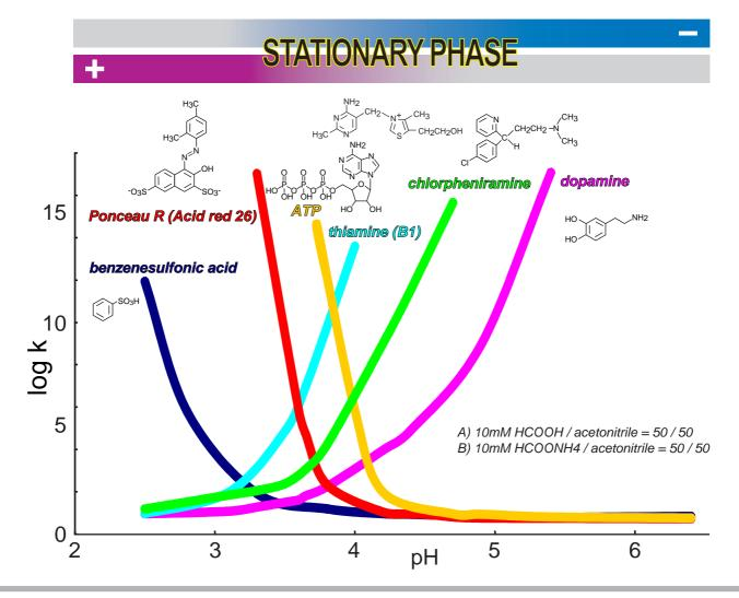
The Nardis ND-NX column incorporates both anion and cation ion ligands. These charged ligands enable electrostatic interactions, making not only cation exchange and anion exchange possible but also normal-phase mode.
